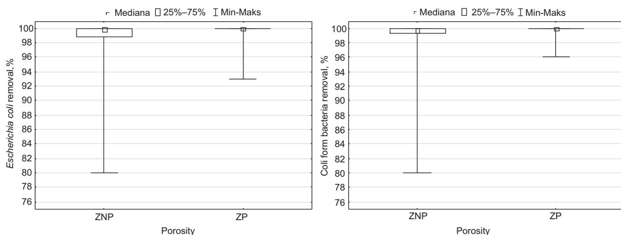
**Fig. 3.** Box-plot graphs of pathogenic bacteria removal on beds filled with porous (ZP) and non-porous material (ZNP)
