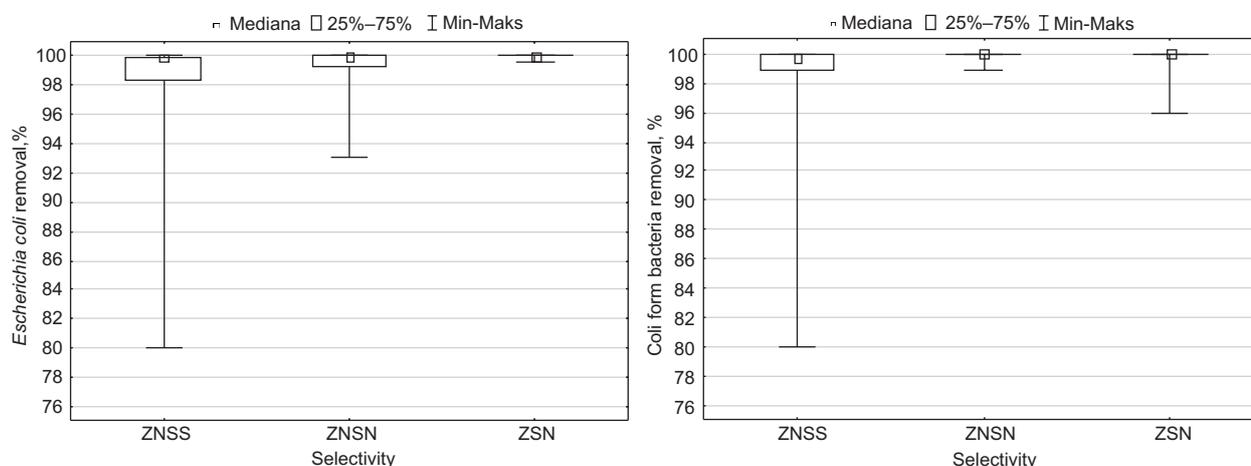
**Fig. 5.** Box-plot graphs of pathogenic bacteria removal on beds filled with non-selective plastic (ZNSS) and natural (ZNSN) material or selective natural material (ZSN)
