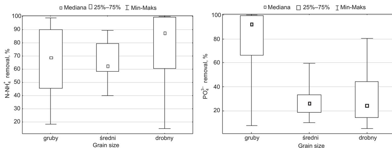
**Fig. 6.** Box-plot graphs of biogenic compounds removal on beds filled with coarse, medium and fine material
