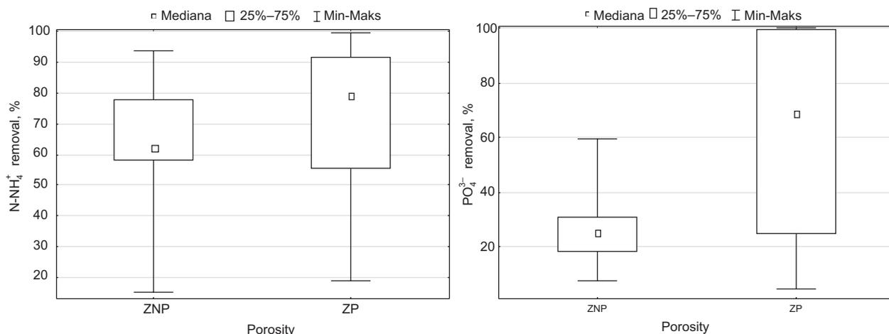
**Fig. 2.** Box-plot graphs of biogenic compounds removal on beds filled with porous (ZP) and non-porous material (ZNP)
