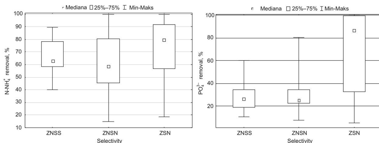
**Fig. 4.** Box-plot graphs of biogenic compounds removal on beds filled with non-selective plastic (ZNSS) and natural (ZNSN) material or selective natural material (ZSN)
