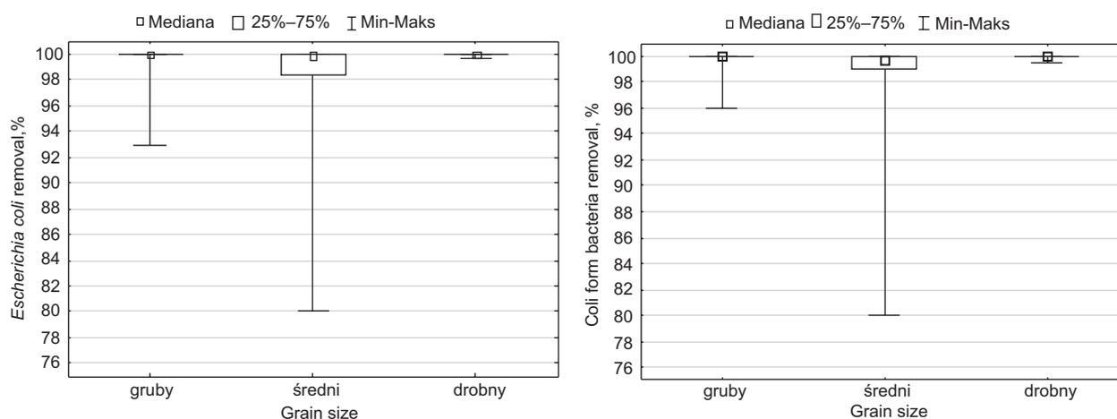
**Fig. 7.** Box-plot graphs of pathogenic bacteria removal on beds filled with coarse, medium and fine material
